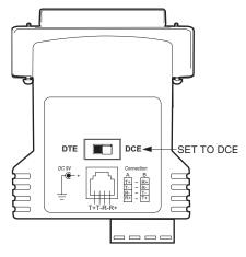
Figure 6. Bottom View of the RS-422 Converter
